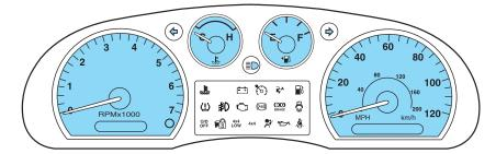
**Speedometer:** Indicates the current vehicle speed.
